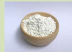
Flux calcined Diatomaceous Earth for filler in paints and as Filter aid.
